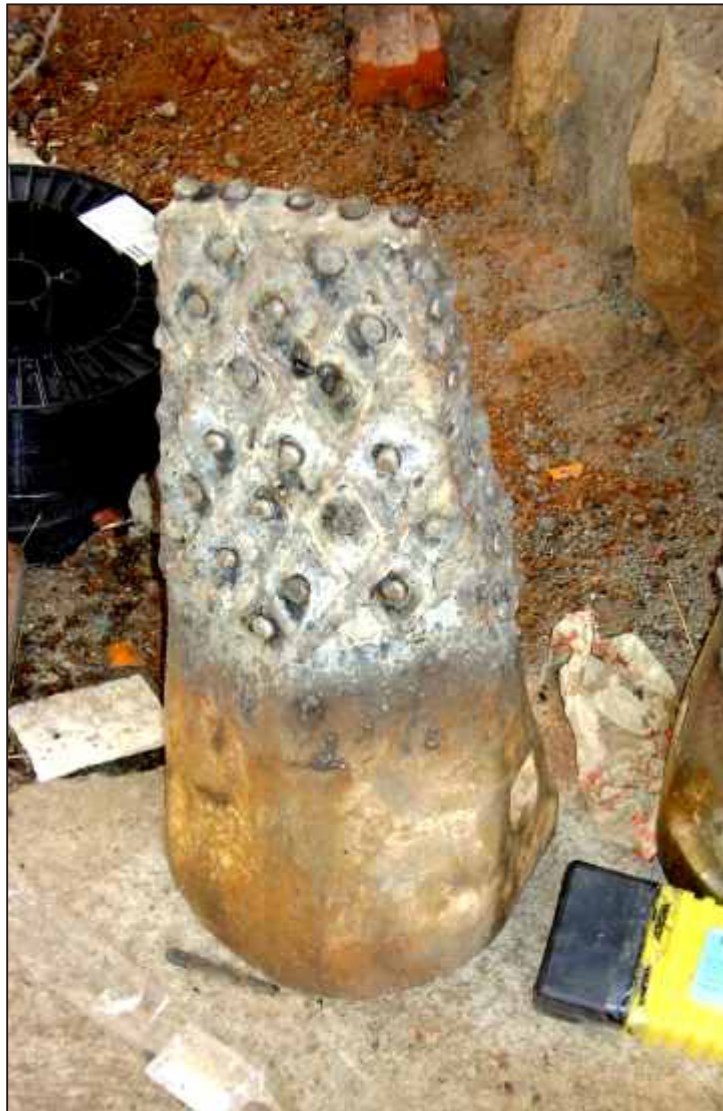
The repaired Tooth Point of PC 3000 Bucket
