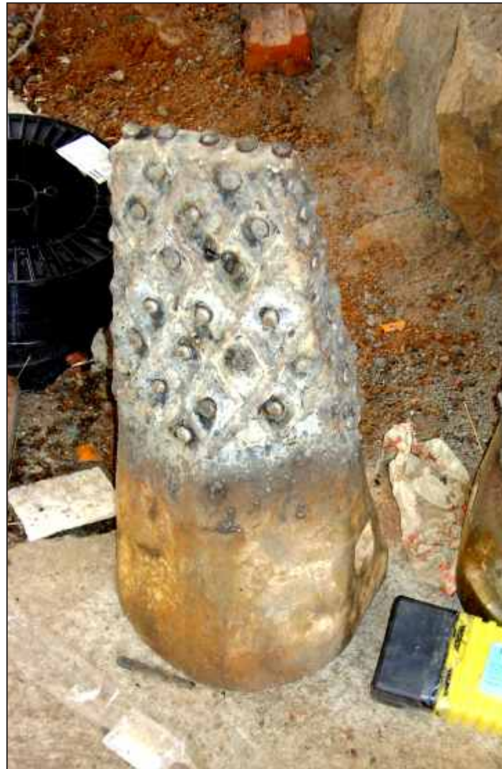
The repaired Tooth Point of PC 3000 Bucket
